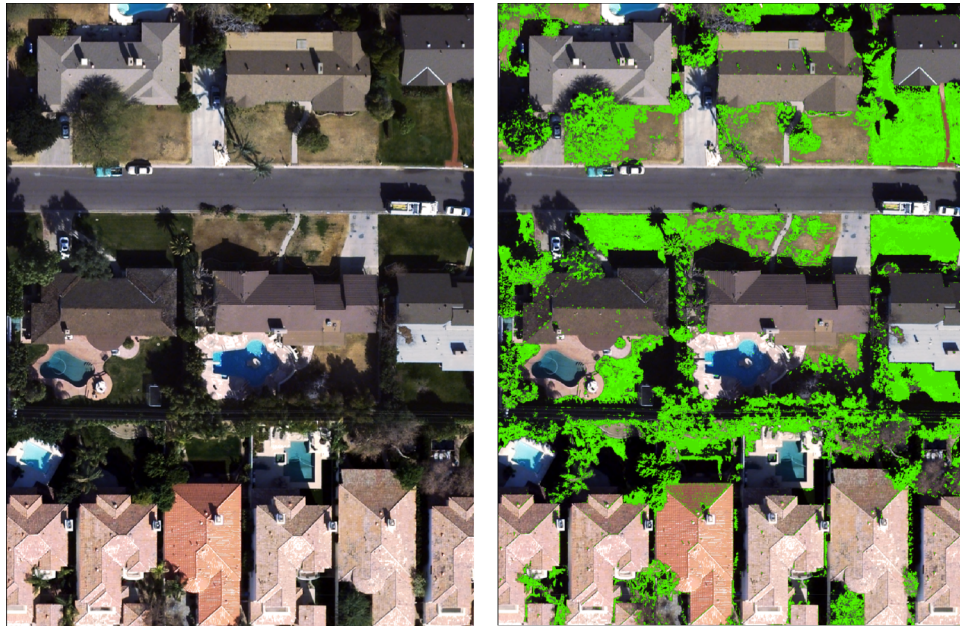
Figure 2: Illustrative remote sensing images demonstrating the classification of green space. Panel A on the right shows what our remote sensing images look like, while Panel B on the left shows how the machine learning algorithm codes the pixels of green space.
