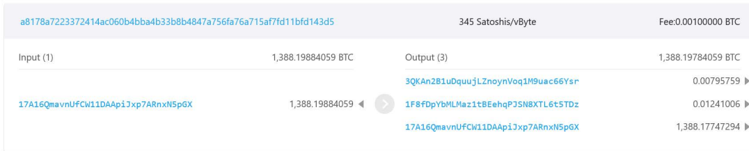
Figure 1: Bitcoin transactions and spurious volume. The figure shows an example of a typical transaction on the Bitcoin blockchain with large spurious volume. The address “17A16Q...” on the left of the ledger, the sender, sends its entire balance to three addresses. The last recipient address that received the majority of the bitcoins is the same as the sending address.
